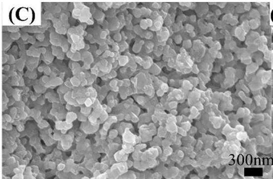
Cross-section of the ScSZ dead-end tubular support sintered at  $1000^\circ\text{C}$
