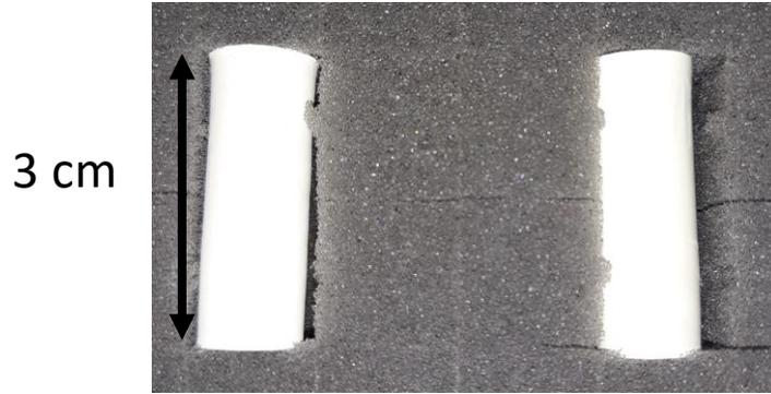
ScSZ-MC dead-end tubular membrane fabricated at USC
