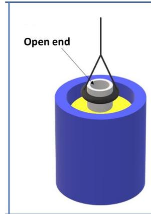
Direct infiltration of molten carbonates at  $600^\circ\text{C}$
