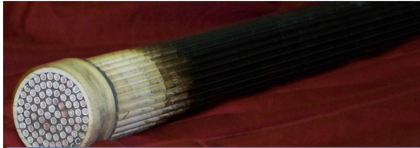
CMS for H 2 Recovery in “Dirty” Gas Systems
