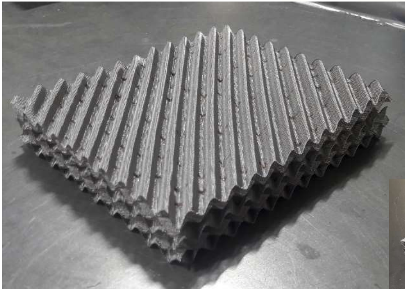
Novel Packing Material for RPB manufactured by Montz (Low Density)
