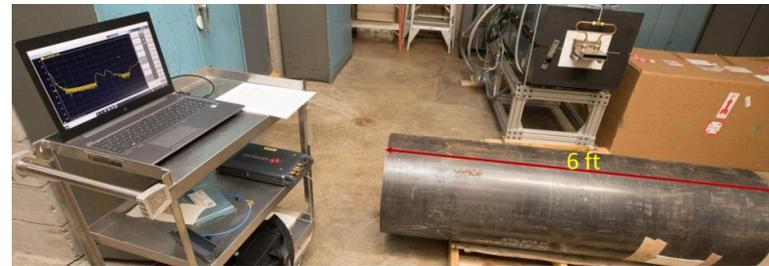
Wireless Interrogation of SAW Sensors Inside Metal Pipe from >1m was Demonstrated.
