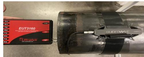
Magnetostriction Acoustic Actuator: 20-30kHz
