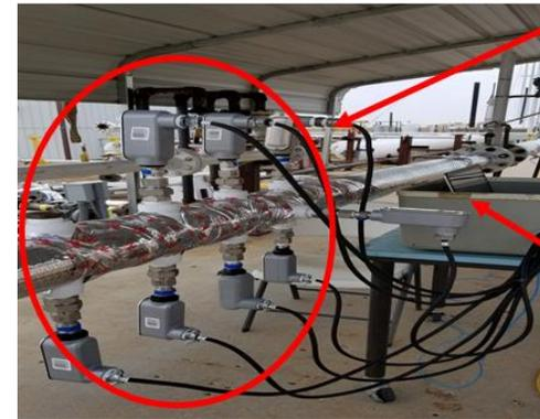
2<sup>nd</sup> generation AES during testing in water-saturated natural gas at CEESI multi-phase flow facility.
