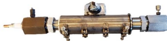
Catalytic Non-Thermal Plasma (CNTP) reactor developed in collaboration with Susteon
