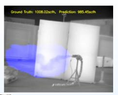
Methane Leak detected from aerial platform
