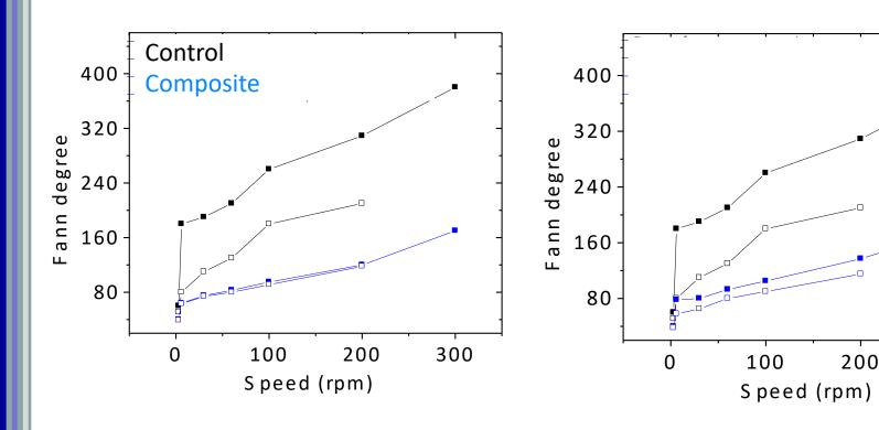
Ramp up and down coincide in composite slurries → no segregation
