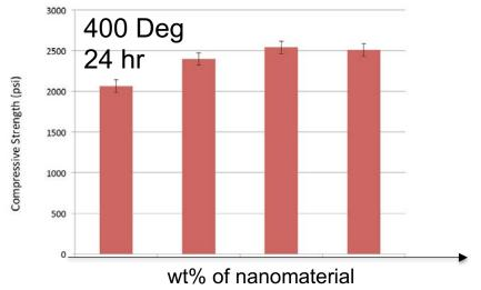
Significantly higher thermal tolerance vs control sample
