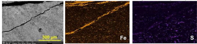
Barium ions + sulfate from breaker = abundant barite precipitation via SEM/EDS
