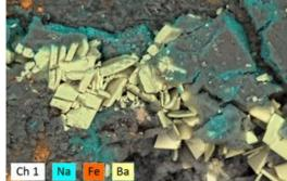
Acid + carbonate-rich mineralogy = significant dissolution via SEM/EDS
