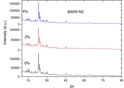
XRD of Mo/ZSM-5 with different loading after MW exposure at 600W
