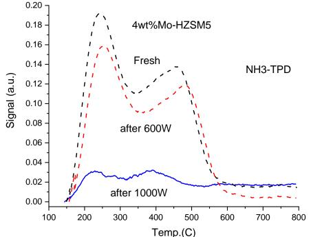
Acid properties of Mo/ZSM-5 (4wt% Mo) exposed to different MW powers (0, 600 and 1000W)
