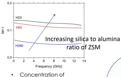
Concentration of surface hydroxyl groups affects the MW absorption of zeolite
