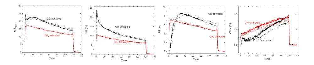
CO activation of Mo catalyst gives higher yields compared to methane activation (likely to reduced carbon formation during activation)
