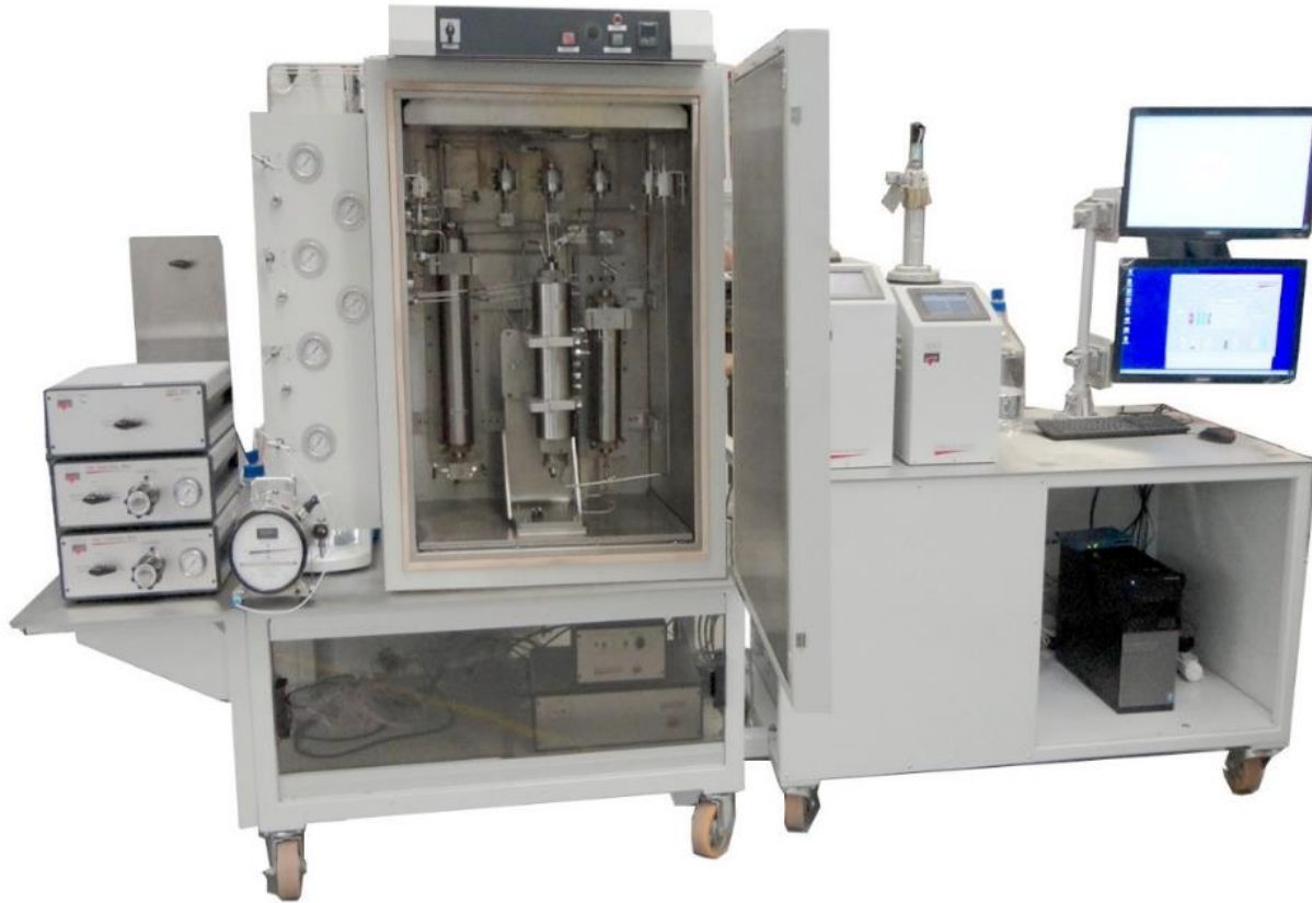
Vinci Core Flood System Used for CO 2 /C2/C3 Injection
