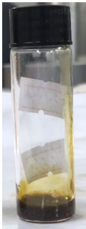
C2-Flooded Oil, additional 1 mL after CO 2 flood
