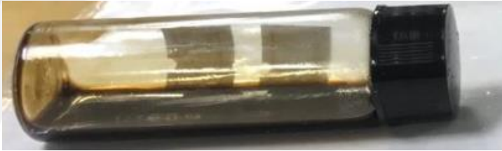
CO 2 -flooded oil; oil can flow under room temperature.
