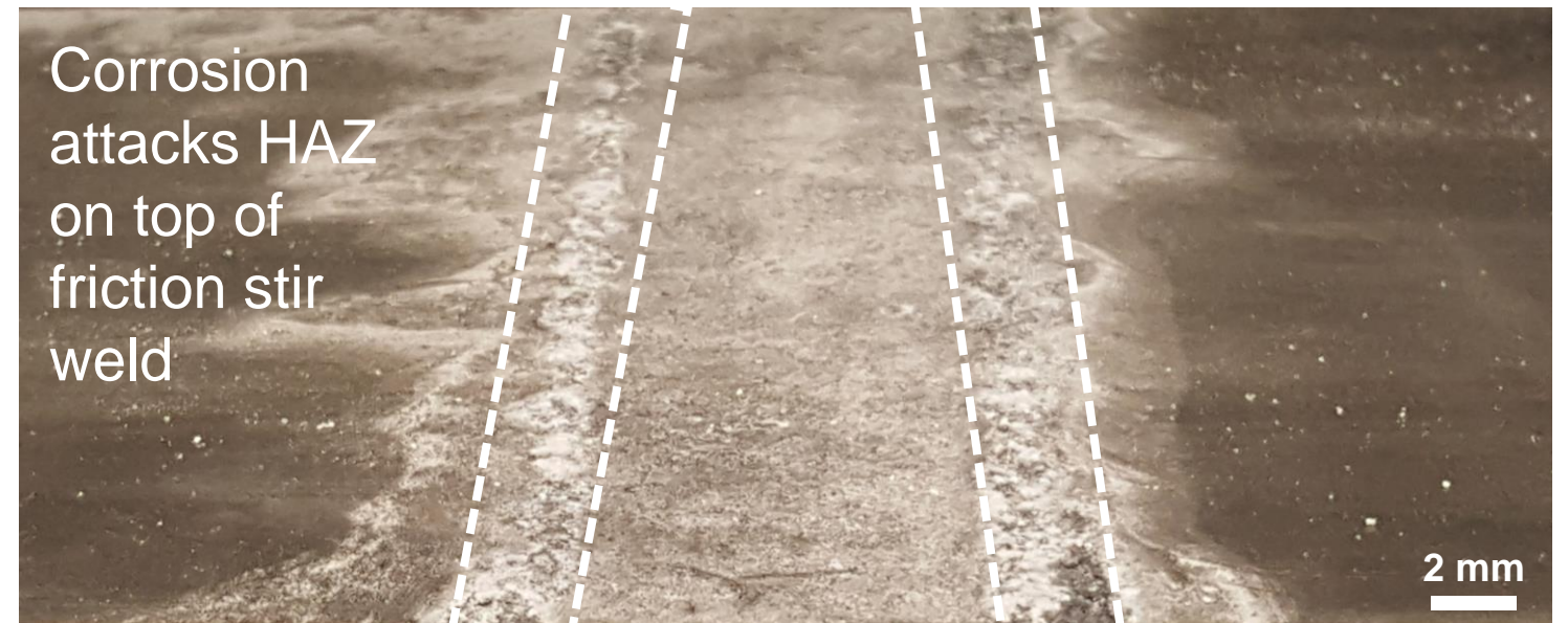
Simulated seawater corrosion testing per ASTM G31-12a and D1141-98
