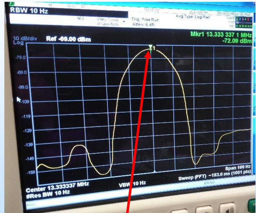
**Measured 13.33 MHz output tone of -72.09 dBm for a 40 MHz input of 3 V<sub>pp</sub>**
