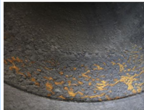
Different form of internal corrosion in natural gas pipeline **
