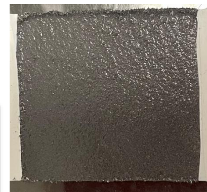
Full size pulse-deposited Pb-GDE
