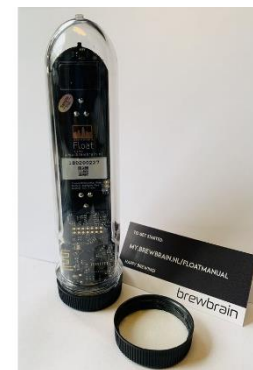
Digital Wifi hydrometer for continuous density readings
