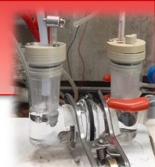
Direct H-cell studies with a Pb wire cathode
