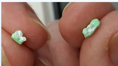
Extruded pellet support with catalyst coating
