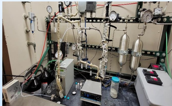
Adsorbent Catalytic Reactor (ACR) Test Unit
