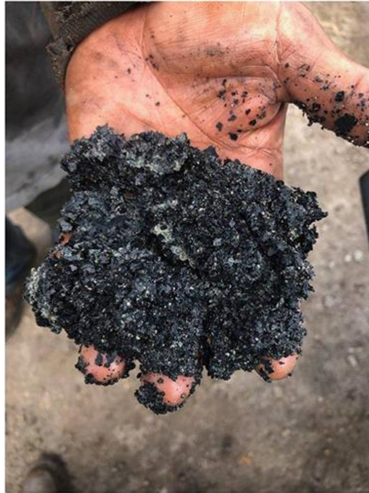
Debris cleared from well during screen/well development
