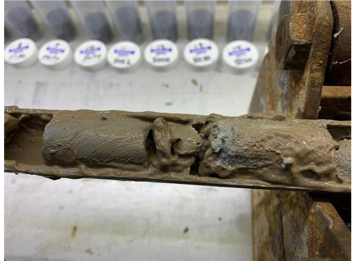
Close-up view of side-wall cores Clay (left) and sandstone (Right)
