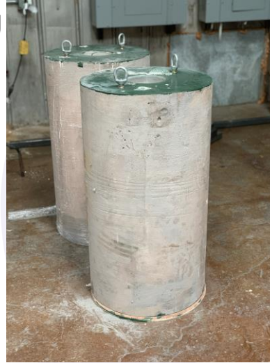
Mancos Shale cores - CT scans
