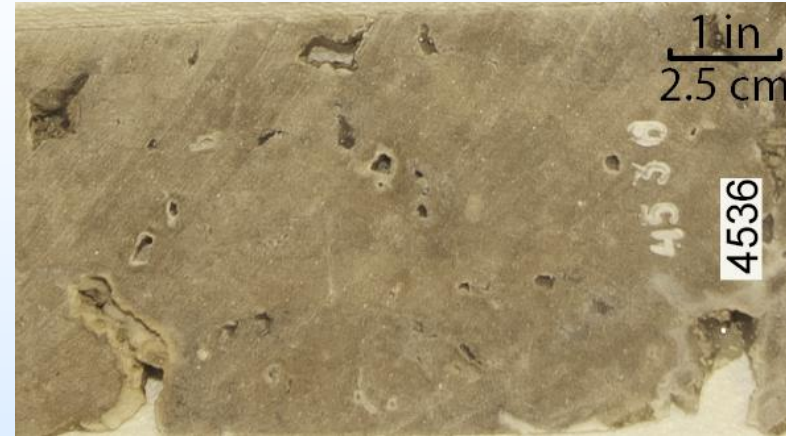
Vuggy porosity with the cavities lined with drusy quartz in the Potosi Dolomite; ADM Verification Well #1, Macon Co. IL.
