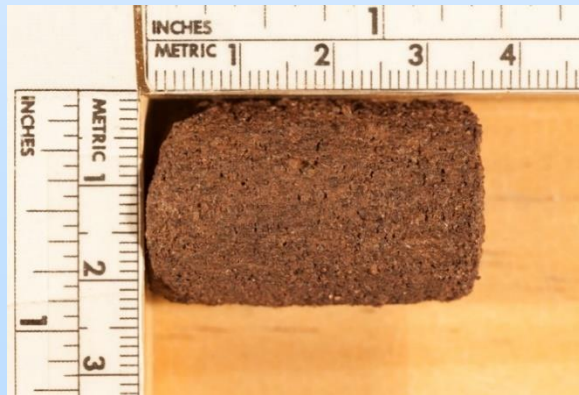
Rotary sidewall core plug from 8690 ft MD
