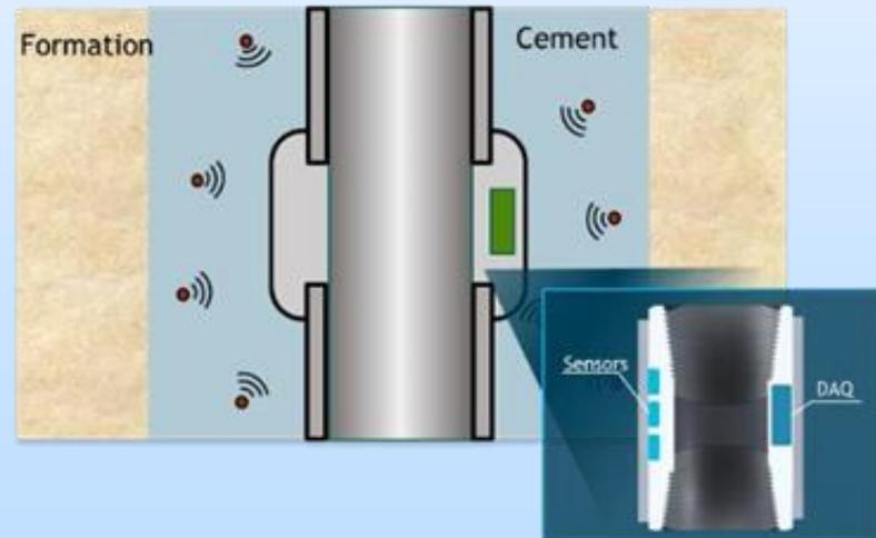
(Left) Sensor systems that communicate wirelessly with casing collars, (Right) providing real-time distributed sensor measurements in the casing annular space, and the formation
