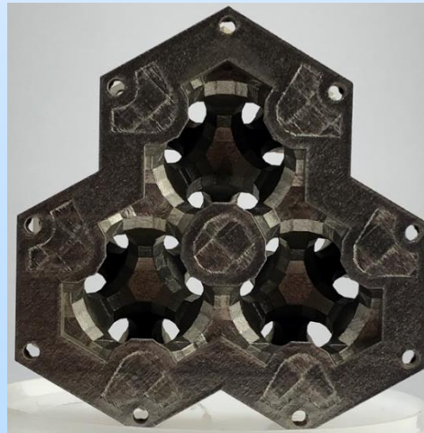
As made and MOF-binder composite-coated 3D contactor components.
