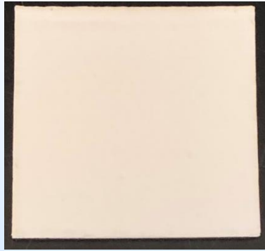
2" x 2" MOF-binder composite coated coupon
