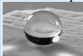
Hydrophobic aerogel monolith
