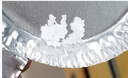
Polyamine film Approx. 1 mm thick
