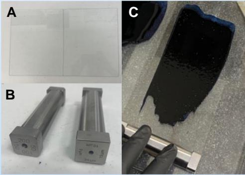
**Figure:** Methods and materials for active polymer layer casting: (A) large 8" by 10" glass substrates, (B) doctor blades, and (C) freshly cast active polymer layer
