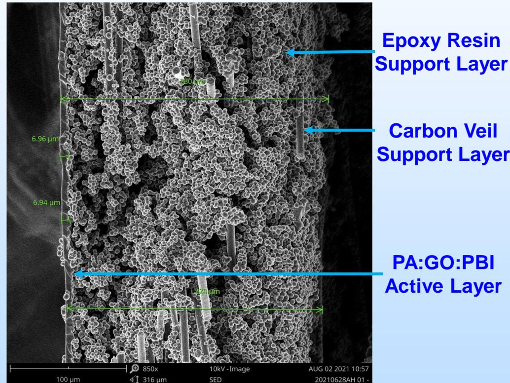
Figure: SEM image of a cross sectional PA:GO:PBI HypoMem sample.
