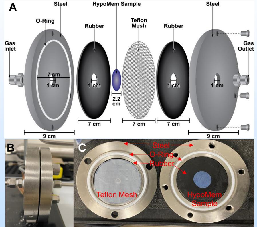
**Figure:** The component parts of the permeation cell at ISL: (A) Exploded view of the permeation cell; (B) Closed permeation cell; and (C) Open permeation cell showing components.
