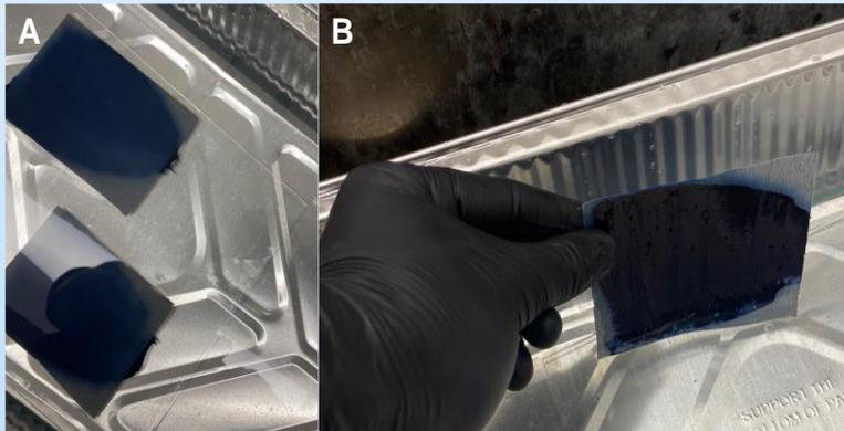
**Figure:** Thin-film lift off method (T-FLO) with HypoMem samples: (A) Submerged in water; and (B) Lifted off the large glass substrate.
