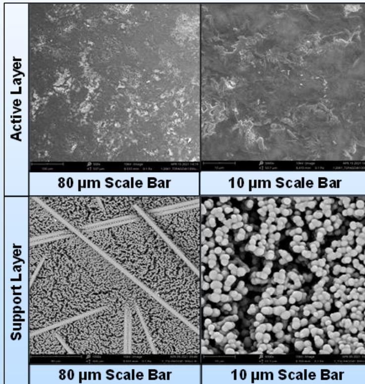
Figure: SEM analysis of a PA:GO:PBI HypoMem sample.
