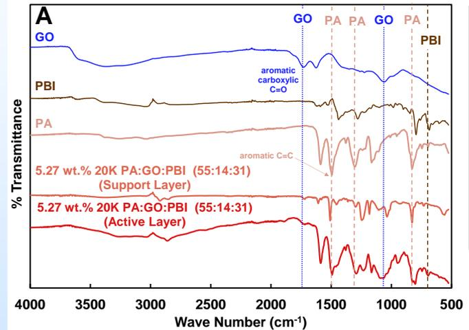
**Figure:** Observed characteristic FTIR peaks of PA, PBI, and GO in a HypoMem sample
