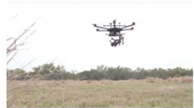
SLED/M Methane Plume Detection (red) of a plume that cannot be readily seen on the MWIR camera (upper photo). SLED/M mounted on a drone platform for aerial, real-time methane leak detection (lower photo).
