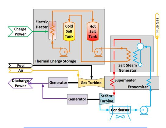
Potential Retrofit to Existing Simple Cycle Fleet to Boost Flexible Capacity using Renewable Power
