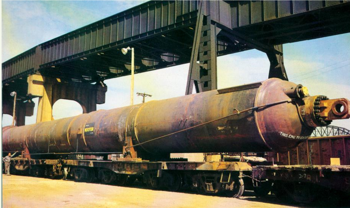
96-ft Long High-Pressure Steel Vessel for ammonia conversion manufactured in the US in 1970s
