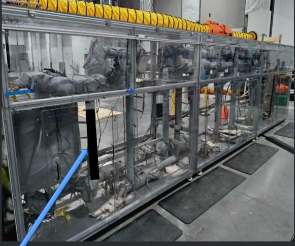
View of test space for sCO<sub>2</sub> pyrolysis loop.
