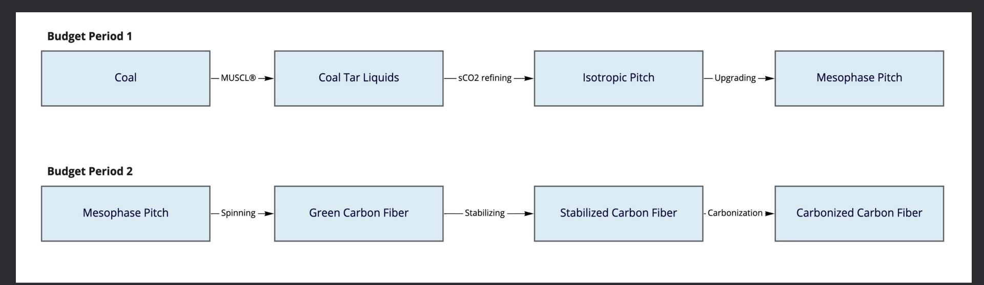
Main technical focus area is on the supercritical CO<sub>2</sub> processing steps.
