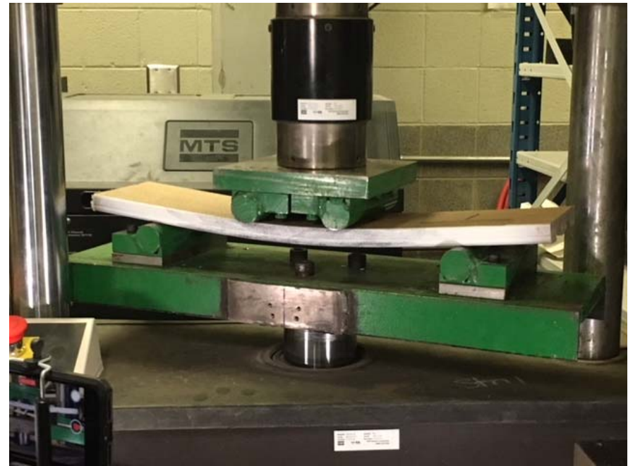
ASTM D1609 Four-point Bend Test (CPC Board Shown)
