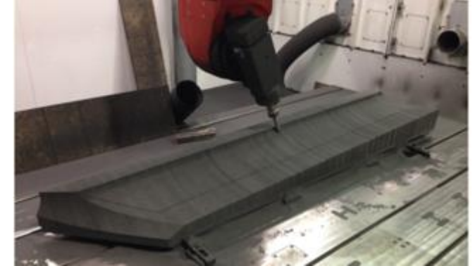
CFOAM carbon foam winglet machining
