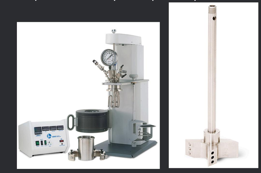
1L Parr Reactor, Gas Entrainment Impeller, and Solids Charging Port (expected delivery 4/30)
