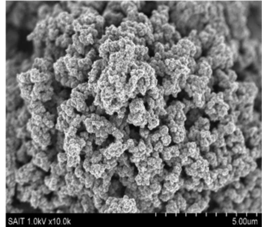
Samsung's "**Graphene Ball**" for Li ion batteries with up to **5x faster charging speed** and **45% more capacity**.
