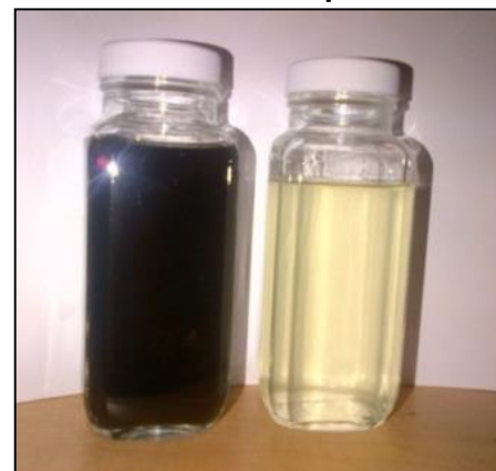
Produced Water (Inlet), Condensed steam (Outlet)
