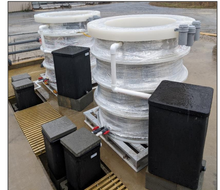
Field lysimeters connected to runoff and leachate tanks
