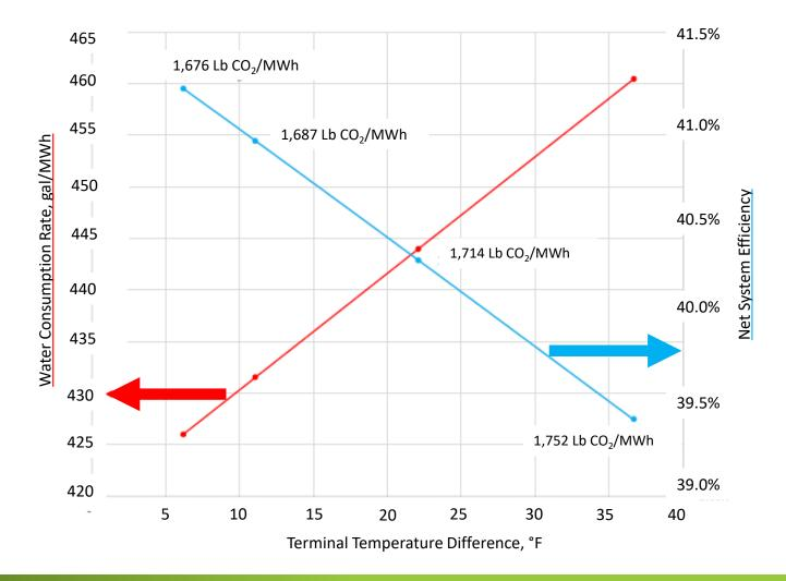
Condenser improvement example: as terminal temperature difference  $\downarrow$ , CO<sub>2</sub> emissions and water consumption rates  $\downarrow$
