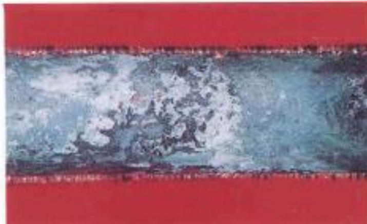
General corrosion inside copper tube because of \text{CO}_2
