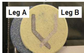
Thermocouple deposited on a furnace cycle test button.
