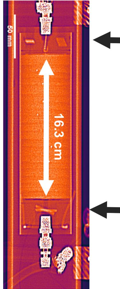
Endcaps with Al coupons for measuring endcap movement
