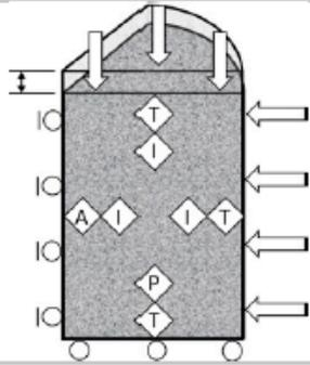
Summary: Vertical consolidation of a single, cylindrical grid cell. Homogeneous system.
