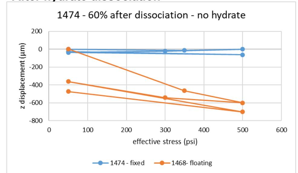
Piston shift (µm) for different experimental conditions
