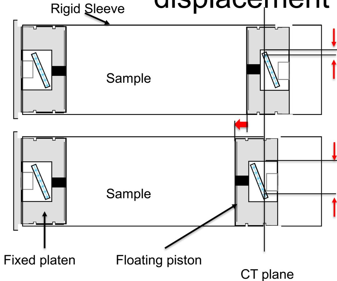
Use slanted X-ray visible coupon in platen and piston
