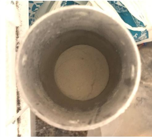
1. Ice was made by freezing water droplets over liquid N2
