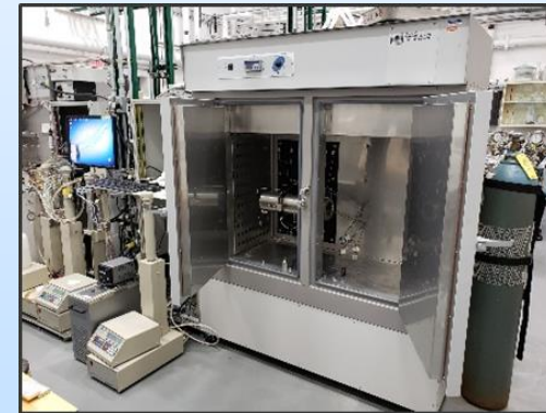
Coreflood setup for confined Huff n' Puff
