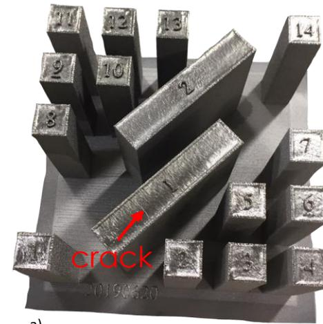
Very different crack pattern compared to CM247
