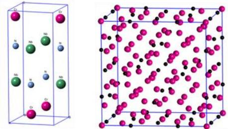
DFT and CALPHAD used to optimize alloy composition. Simulations used to determine the effect of alloying elements on the formation and stability of unwanted (Z-phase) and desired strengthening phases (Carbides).
