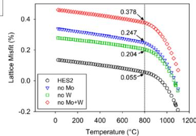
Alloy 282: Increase the gamma prime fraction/solvus to enhance >800C mechanical properties. Obtain a gamma prime fraction/solvus at 900C equal to that of the commercial alloy at 800C. Also looking at Alloy 263 and Nimonic 105.
