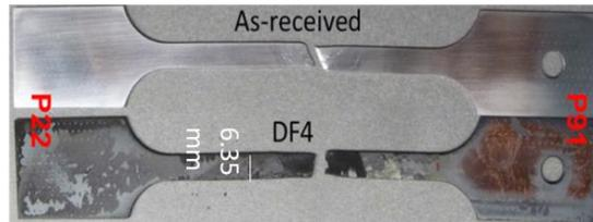
Exposure to CO<sub>2</sub>+4%H<sub>2</sub>O+1%O<sub>2</sub> (DF4) for 1000h
