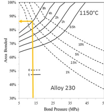
Strength of the bonded stacks was greater than 85% of base alloy 230 yield stress. Bonded stacks possessed acceptable low-cycle fatigue and creep properties. However, plastic strain localization in the bond region caused low tensile and creep elongation
