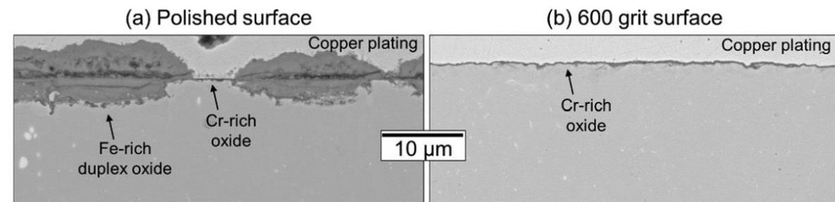
Pure CO<sub>2</sub> – repeating experiment under direct cycle environments
