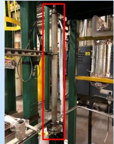
The first 19-membrane module with total membrane area of  $0.13 \text{ m}^2$  installed in UK CAER's large bench unit.
