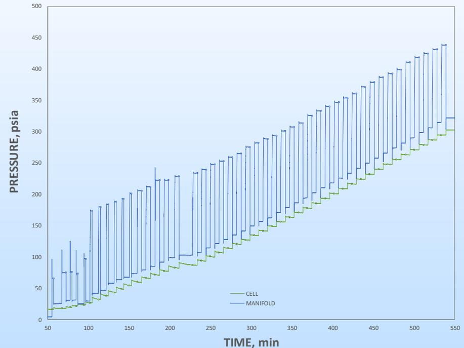
PTxy Injection Profiles at 40°C MDEA/PZ/H<sub>2</sub>O (45:5:50w/w)
