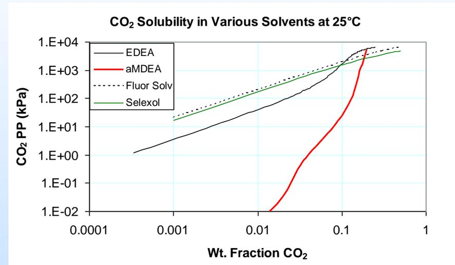
Anhydrous EDEA absorbs CO<sub>2</sub> stronger than physical solvents but weaker than chemical solvents.
