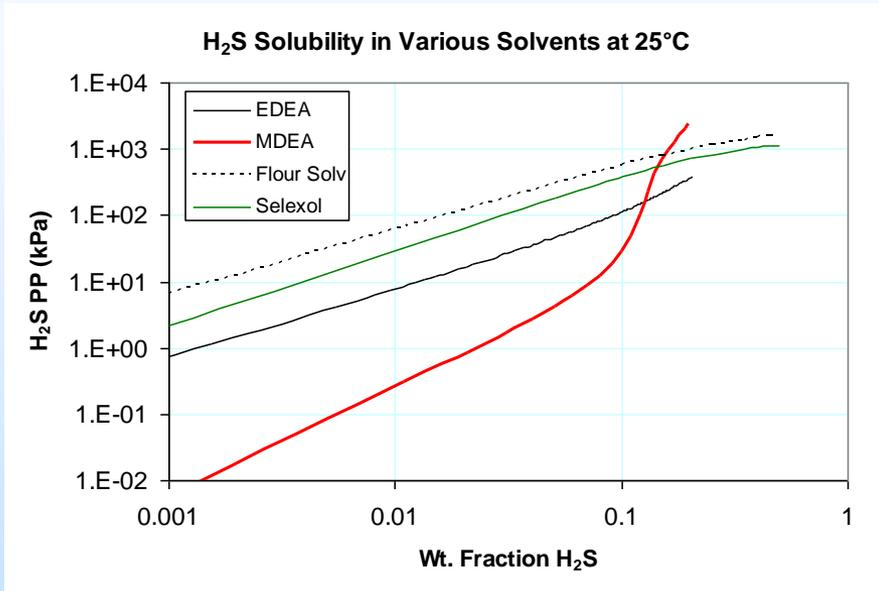
Anhydrous Ethyldiethanolamine (EDEA) absorbs H<sub>2</sub>S more strongly than physical solvents but weaker than chemical solvents.
