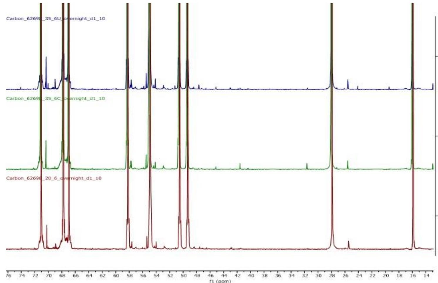
Representative comparison of  $^{13}\text{C}$  NMR spectra of degradation of 2-EEMPA during reaction 6. Top: with uncoated 316 SS chips, middle: with Silcotek<sup>®</sup>-coated 316 SS chips, bottom: in the absence of 316 SS. Similar NMR spectra were recorded for 30 wt.% MEA.
