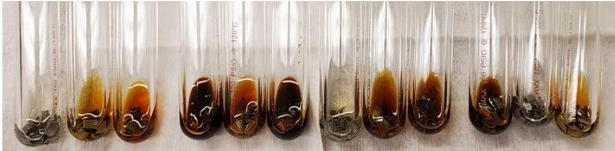
Visual comparison of different samples of oxidatively-degraded 2-EEMPA. Similar visual assessments were observed with 1-IPADM-2-BOL and 30 wt.% MEA.
