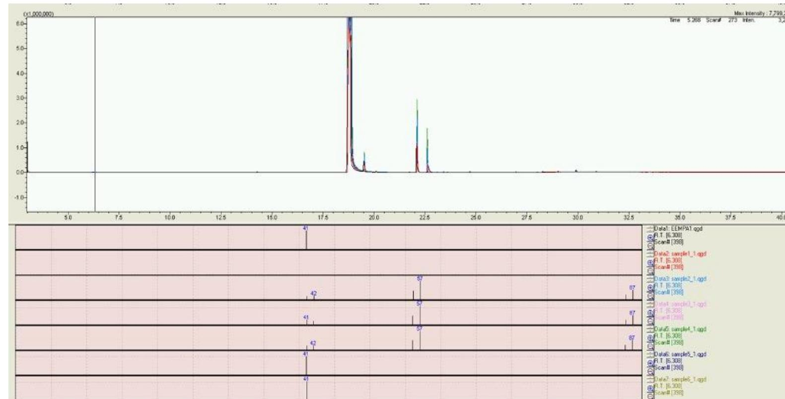
Representative stacked MS analyses' results of reactions of 2-EEMPA. Similar MS analysis was performed for 30 wt.% MEA.
