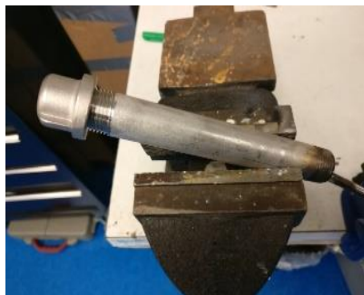
Sensor packaged in 6" long closed tube
