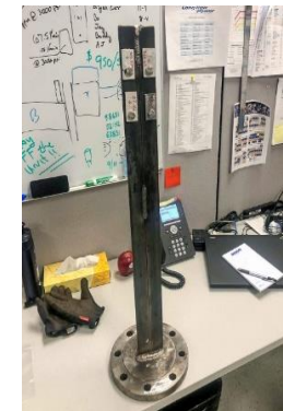
FIRST: Four coated low-carbon steel coupons installed
