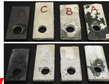
FIRST: Four coated low-carbon steel coupons installed
