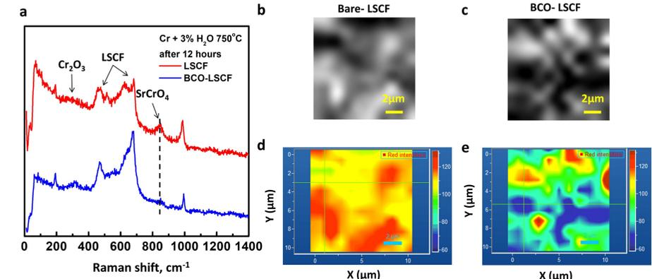
**Figure 5** (a) Typical Raman spectra from a bare LSCF and a BCO-LSCF dense pellet after the Cr poisoning test (3% H<sub>2</sub>O, 750 °C, 12 h); Optical image of bare LSCF (b) and BCO-LSCF (c) for Raman mapping; Raman mapping of -CrO<sub>4</sub> (peak at ~850 cm<sup>-1</sup>) observed from the bare LSCF (d) and BCO-LSCF (e) dense pellet surface after the Cr poisoning test.
