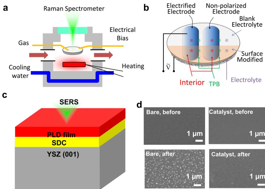
**Figure 2** (a) Schematic for the experimental setup for *in-situ* Raman spectroscopy coupled with electrochemical characterization; (b) critical surface and interface regions in the *in operando* study of electrode behavior; (c) schematic of pulsed laser deposition (PLD) thin film for in situ Raman study; (d) SEM of fresh films and films after Raman testing in conditions with contaminations.
