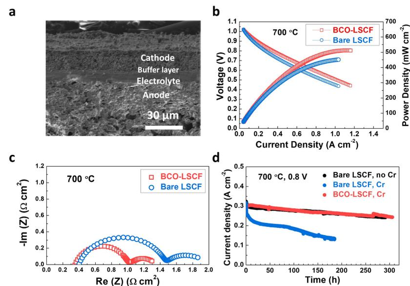
**Figure 4** (a) A Typical cross-sectional SEM image of a Ni-YSZ anode supported cell; (b) Typical I-V-P and (c) EIS curves of the cells with a bare LSCF or BCO-LSCF cathode at 700 °C in direct contact with Crofer 22APU; (d) Durability test of single cells with bare LSCF cathode in clean air (black balls), bare LSCF (blue balls), and BCO-LSCF (red balls) in 3% H<sub>2</sub>O-air and a direct Crofer 22APU contact.
