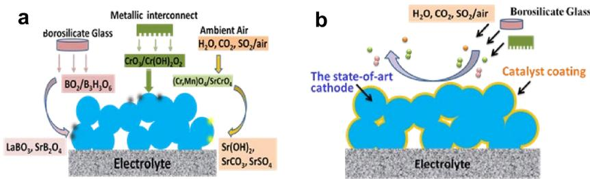
**Figure 1** (a) Schematic diagram showing the sources of volatile Cr, B, and S species, and the respective reaction products on a cathode (b) schematic for a high-performance cathode consists of the state-of-the-art cathode backbone (e.g., LSCF) and a durable catalyst against various contaminants, making effective use of the best properties of two different materials (backbone and catalyst).
