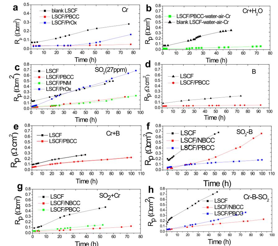
**Figure 6** Interfacial resistance of blank LSCF and catalyst coated LSCF as a function of time, when exposed to different contaminant. (a) in direct contact with Cr in dry air; (b) in direct contact with Cr in 3% H<sub>2</sub>O; (c) 27 ppm SO<sub>2</sub> in air; (d) boron-silicon glass; (e) Cr and B-silicon glass; (f) B-silicon glass and air with 27ppm SO<sub>2</sub>; (g) Cr and air with 27ppm SO<sub>2</sub>; (h) Cr and B in air with 27ppm SO<sub>2</sub>.
