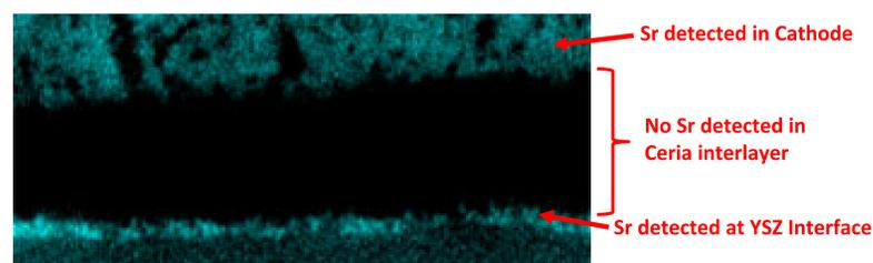
During sintering, Sr from LSCF cathode diffuses to YSZ interface and reacts to form strontium zirconate. A Sr concentration gradient characteristic of solid phase diffusion that would be expected across the ceria interlayer is absent. Could vapor phase transport play a role?
