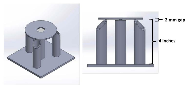
Transport testing was performed using the alumina test setup shown here. A very long surface pathway and small contact points are designed to ensure any transport is happening via the vapor phase.
