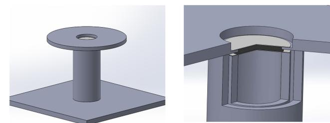
Experiments are underway using the modified alumina test setup shown here. An outer tube now supports the top substrate holder while also enclosing the space where Sr and Co vapor will be present. This will allow the vapor phase species to remain concentrated. The surface pathway is still very long, with a small gap separating the inner and outer support tubes. This ensures any detected transport will have occurred through the vapor phase.
