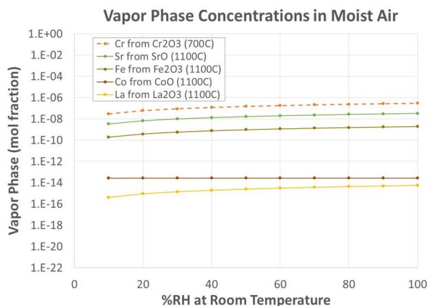
Sr volatility at 1100°C is within an order of magnitude of the level of Cr that poisons SOFC cathodes at 700°C and is the highest amongst LSCF components.
