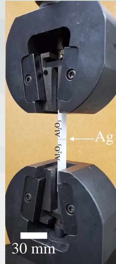
The tensile test sample and experiment set up
