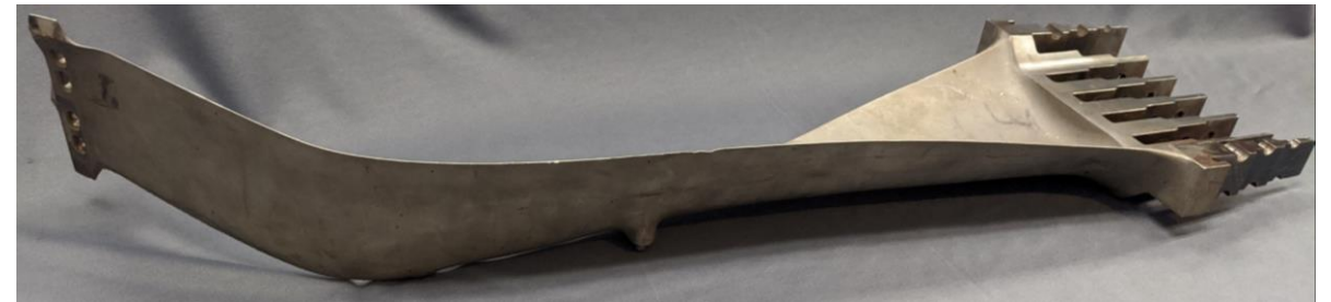
Turbine Blade (damaged) Removed From Service
