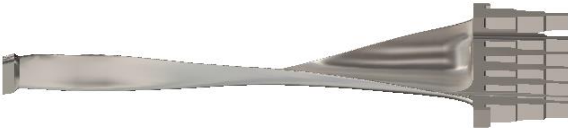
Turbine Blade Solid Model from 3D Point Cloud
