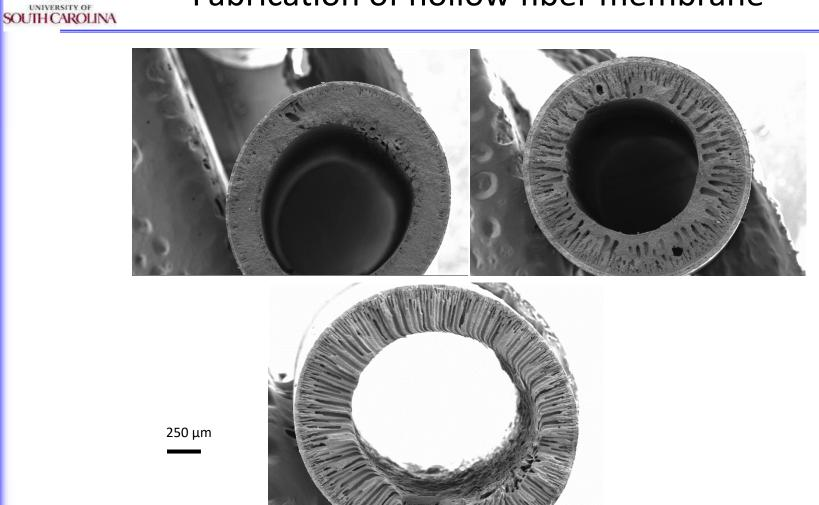
Fabrication of hollow fiber substrates :
