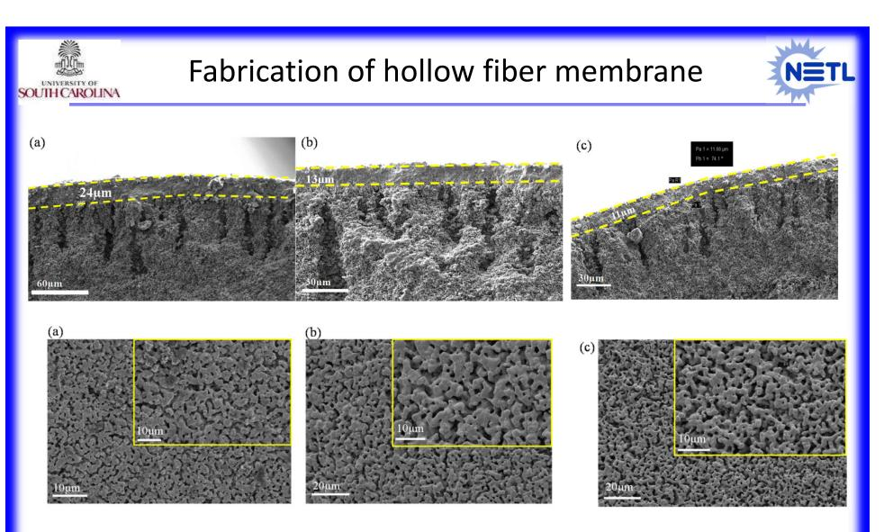
Process optimization of functional layer fabrication
