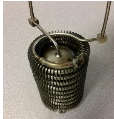
Coiled-fin tube exchanger between dual AMRs
